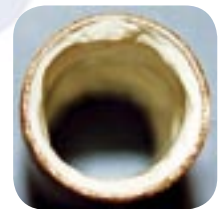
Water pipe with lime scale deposits before.
